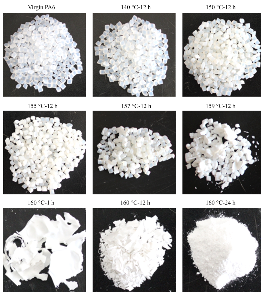
Fig. 2 Morphology of the PA 6 samples recovered from hydrothermal treatment with different conditions (For example, 140 °C-12 h means hydrothermal processing at 140 °C for 12 h.)
